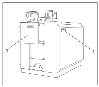
Fig. 42 Hooking on the burner door cover
