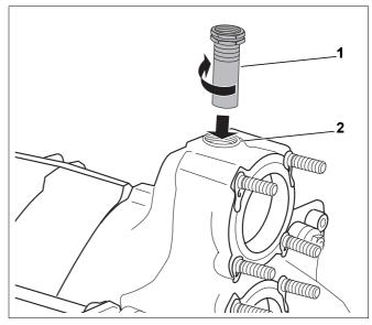
Fig. 20 Sensor well installation
