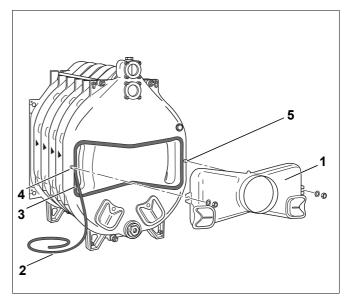
Fig. 24 Flue gas collector installation
