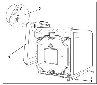
Fig. 35 Side casing installation
