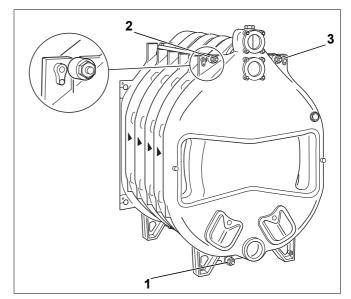
Fig. 17 Installation of the tie bars
