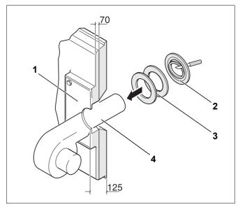
Fig. 28 Burner installation (dimensions in mm)
