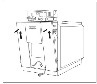
Fig. 54 Remove the front wall
