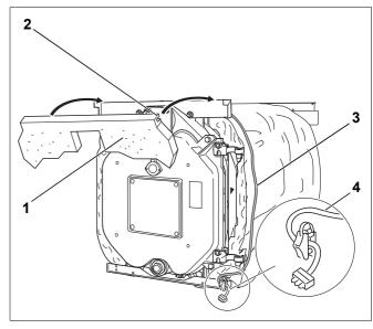
Fig. 34 Installation of the front insulation
