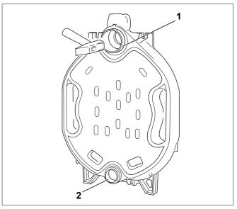
Fig. 9 Hammering the nipples home
