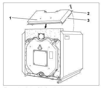
Fig. 36 Installation of the front hood
