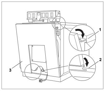
Fig. 41 Front wall installation
