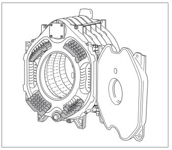
Fig. 27 Hot gas baffle plates
