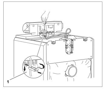
Fig. 47 Securing the electrical connection cables
