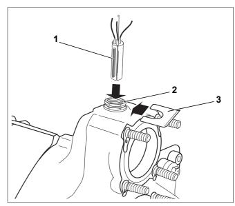
Fig. 45 Sensor bundle installation
