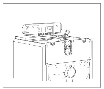
Fig. 48 Boiler with control unit installed
