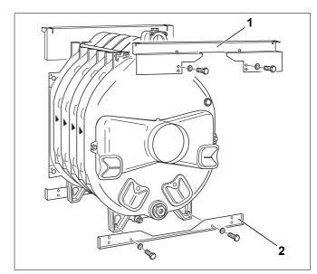
Fig. 31 Installation of the rear support brackets
