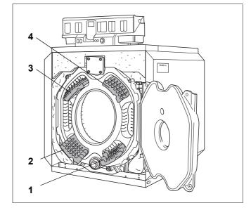
Fig. 55 Remove the hot gas baffles
