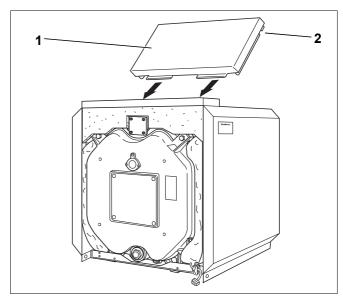
Fig. 37 Installation of the rear hood
