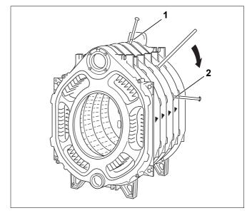
Fig. 22 Separating the boiler block
