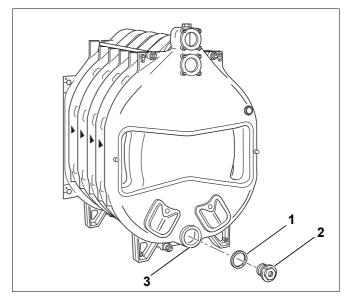
Fig. 21 Flange installation
