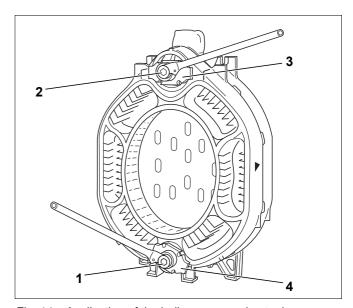
Fig. 14 Application of the boiler compression tool
