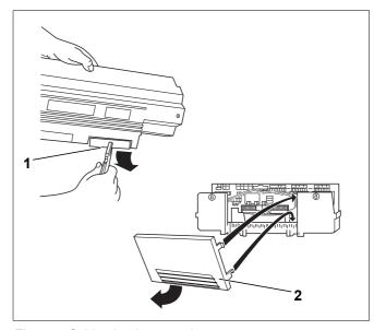
Fig. 44 Cable gland preparation
