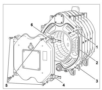
Fig. 26 Hooking on the burner door
