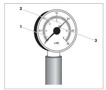
Fig. 60 Pressure gauge for open systems
