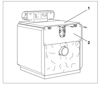
Fig. 39 Installation of the upper boiler back wall
