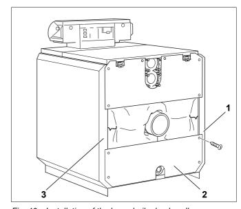
Fig. 40 Installation of the lower boiler back wall
