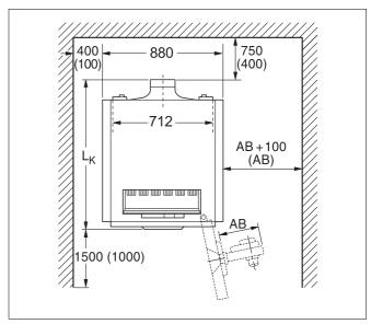
Fig. 4 Boiler room with boiler in place [mm]
