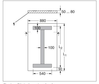
Fig. 3 Plinth dimensions [mm]
