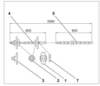
Fig. 2 Boiler compression tool size 2.3
