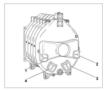
Fig. 25 Rear section with mounted fittings
