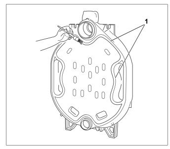
Fig. 10 Coating the packing grooves with adhesive
