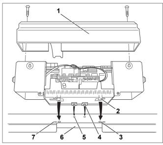
Fig. 43 Control unit installation
