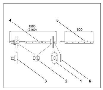
Fig. 1 Boiler compression tool size 2.2
