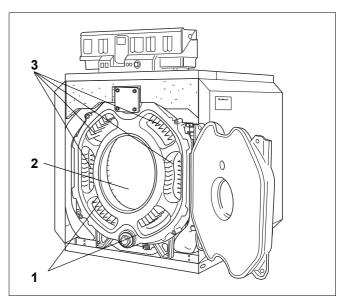
Fig. 58 Cleaning the hot gas flues
