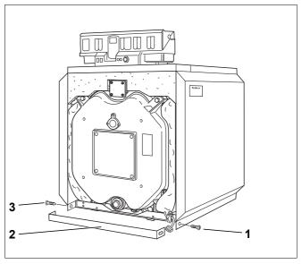
Fig. 38 Installation of the front plinth rail
