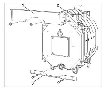
Fig. 30 Installation of the front support brackets
