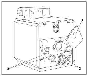
Fig. 56 Cleaning cover removal
