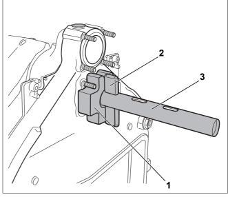
Fig. 15 Boiler compression tool at the rear section
